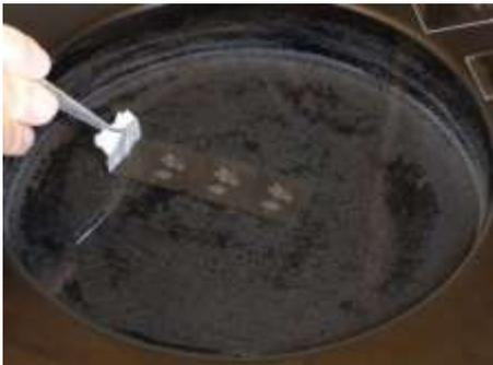
A cut wax/tissue section is gently lifted off the face of the microtome knife edge and floated on top of a water bath. Here three sections from the tissue block can be seen floating on the water (temperature = 50 degrees C)
